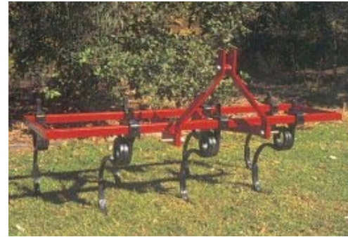
The CT series (coil tynes)
